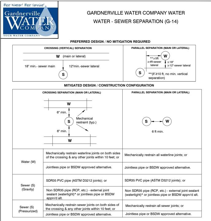
Sewer - (e.g. sanitary sewer mains and laterals, storm drains, and reclaimed wastewater mains and laterals.) Mechanical restraint - a mechanical coupling to restrict joint movement and separation.
