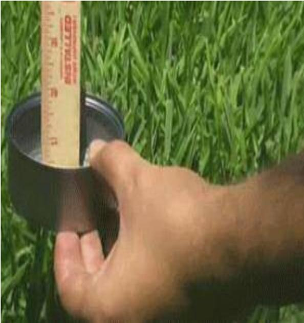
On average, pop-up sprinklers apply 0.4 inches of water in 15 minutes, and impact sprinklers apply 0.2 inches of water in 15 minutes.
